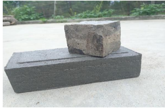
Gambar 10. Sampel Paving Block Plastik (Sumber: Yusuf Amran-Arif Wahyu Permana, 2024)
