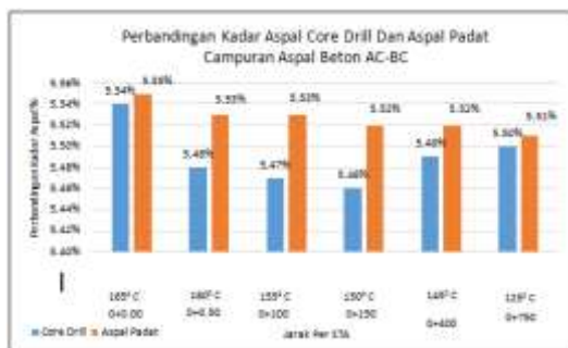
Gambar 1. Perbandingan kadar aspal hasil core drill dan aspal padat campuran aspal beton AC-BC.
