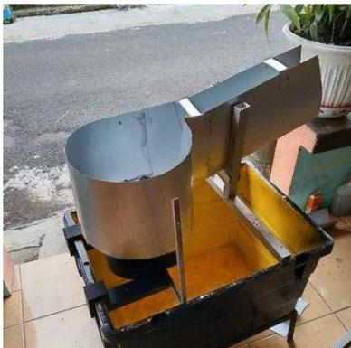
Gambar 3. Instalasi Turbin Vortex
