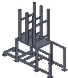
Fig. 2. UNP profile frame with bolt combination.
