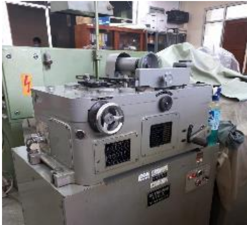
Gambar 9. Ogoshi High Speed Universal Wear Testing Mechne (Type OAT-U).
