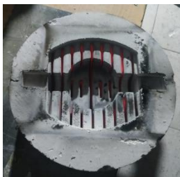
Gambar 4. Hasil pre-heating cetakan
