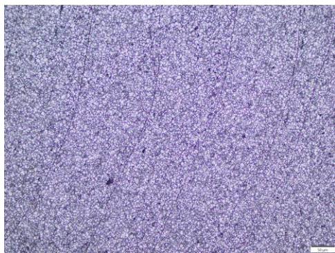
Gambar 6. Foto struktur mikro nugget zone spesimen as welded
