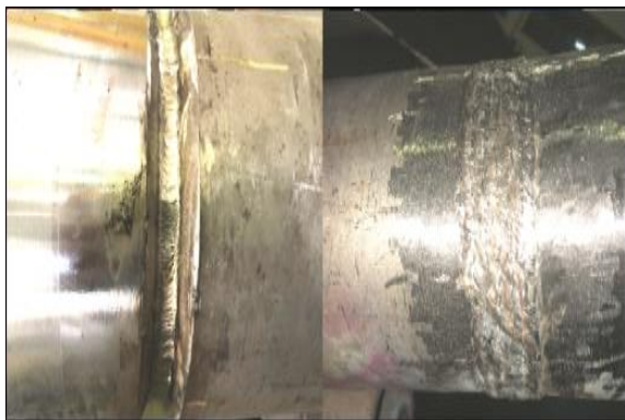
Figure 6. Result of the welding of dissimilar metal SUS 304H and incoloy 800H
