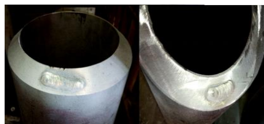
Figure 5. Incoloy 800H weldability test results
