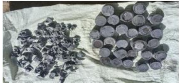
Figure 1. Motorcycle waste piston Preparation of specimen molds made of galvanized pipe with a diameter of 25.4 mm (Figure 2),
