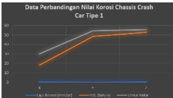
Gambar 11. Nilai Korosi Chassis Crash Car Tipe 1
