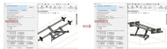
Gambar 11. Hasil reduce of frame weight pada Desain V-Plow Eksisting vs RE ( Reverse Engineering )
