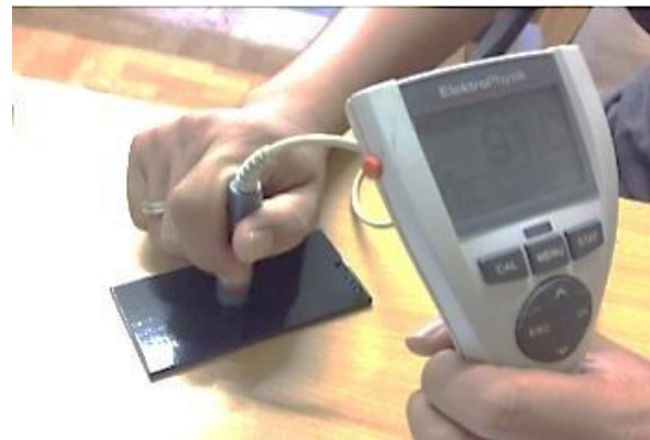
Gambar 2. Pengujian ketebalan lapisan Coating thickness gauge [17]
