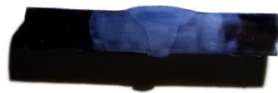
Figure 16. 4 mm Root Gap
