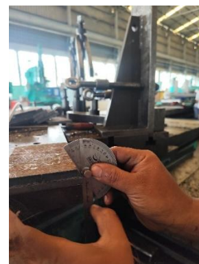
Figure 2. Bevel Angle Formation
