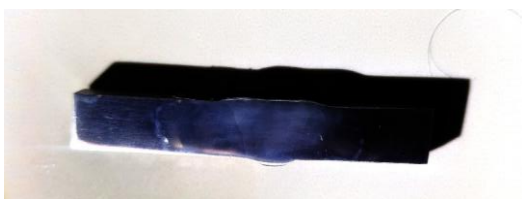
Figure 18. 8 mm Root Gap
