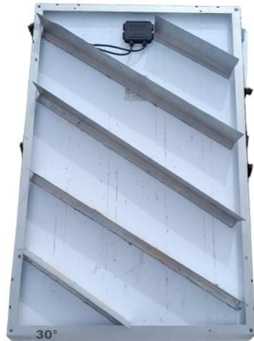
Gambar 2. Panel surya Sudut Sirip 30^\circ
